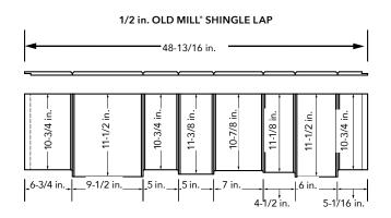
TruWood Old Mill\* Shingle Lap Siding goes up fast and easy. It requires no special tools for installation and it comes in easy to handle 4 ft. lengths and a convenient shiplap edge.
