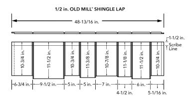
TruWood Old Mill\* Shingle Lap Siding goes up fast and easy. It requires no special tools for installation and it comes in easy to handle 4 ft. lengths and a convenient shiplap edge.
